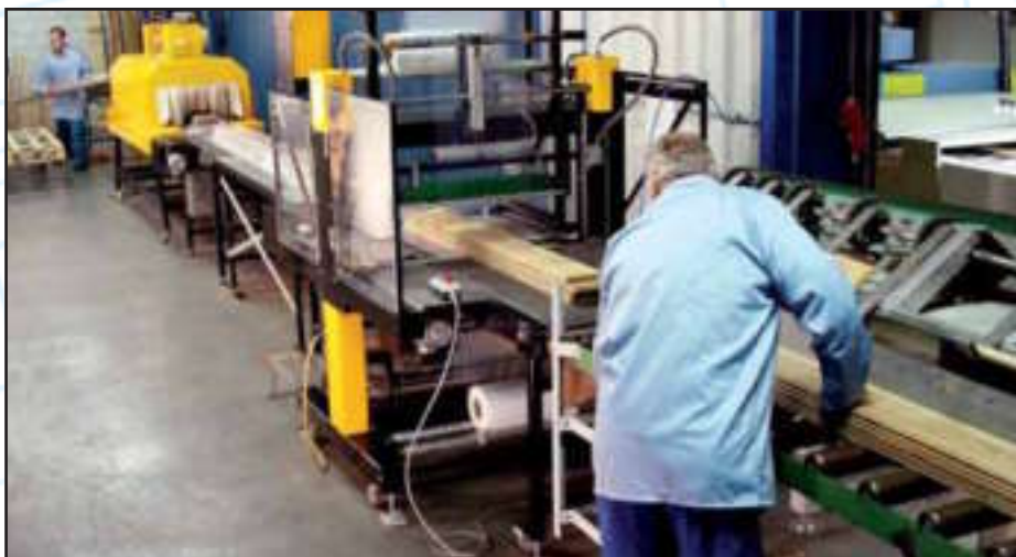
Longer products, such as parquet, require a linear installation.
