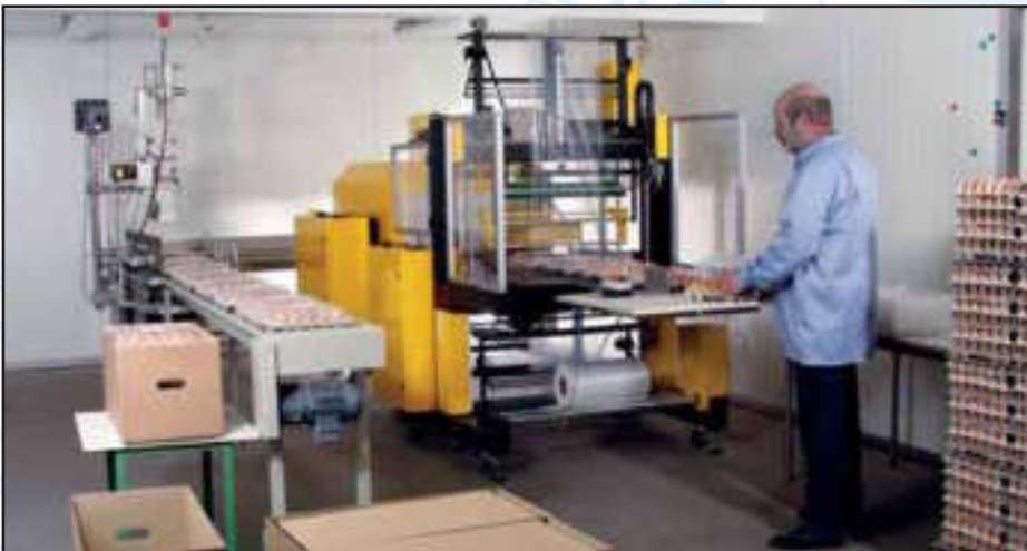
A U-shaped installation permits one-man operation in small spaces.
